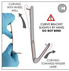
**FIGURE D** Place bracket against wheel well area with the lower portion placed underneath the side skirt as shown. Adjust until the mounting hole is visible through the side skirt mounting hole. Ensure that the foam spacer on the lower portion of the bracket is against the wheel well liner, and uppermost portion of the bracket contours the fender well as shown. Repeat Step C as needed. Upper bracket foam area does not need to touch wheel well.
